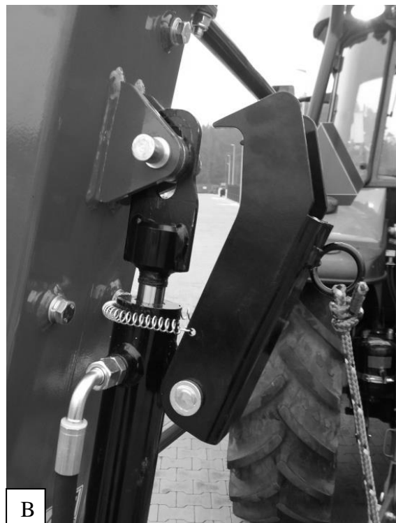
Fig.12 Actuator lock 1 - closed, 2 - open
