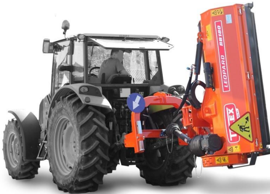
Fig.5 General view of machine in transport position
