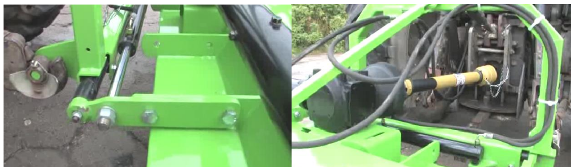
Figure 2. LEOPARD mower – hydraulic shift of the machine
