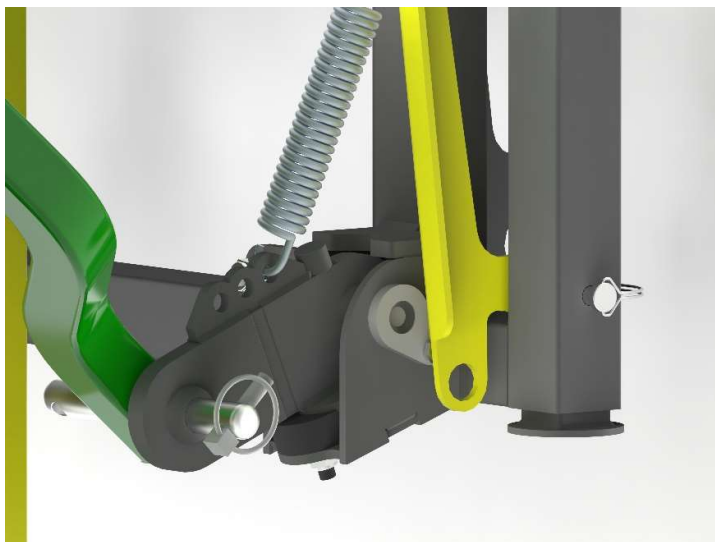
Fig 9 Locking in the working position
