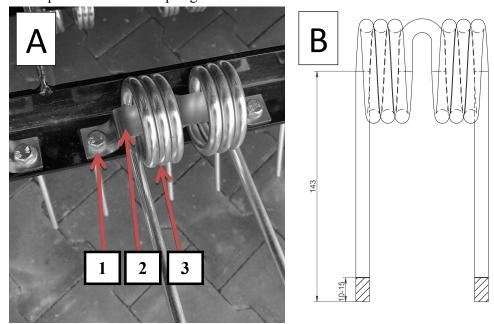
Rys.4. A - Spring protector: 1) protector mounting screw, 2) spring protector 3) spring. B-Acceptable degree of wear of the rake spring.
