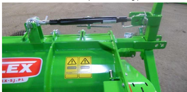
The position of the additional transport hitch during work
