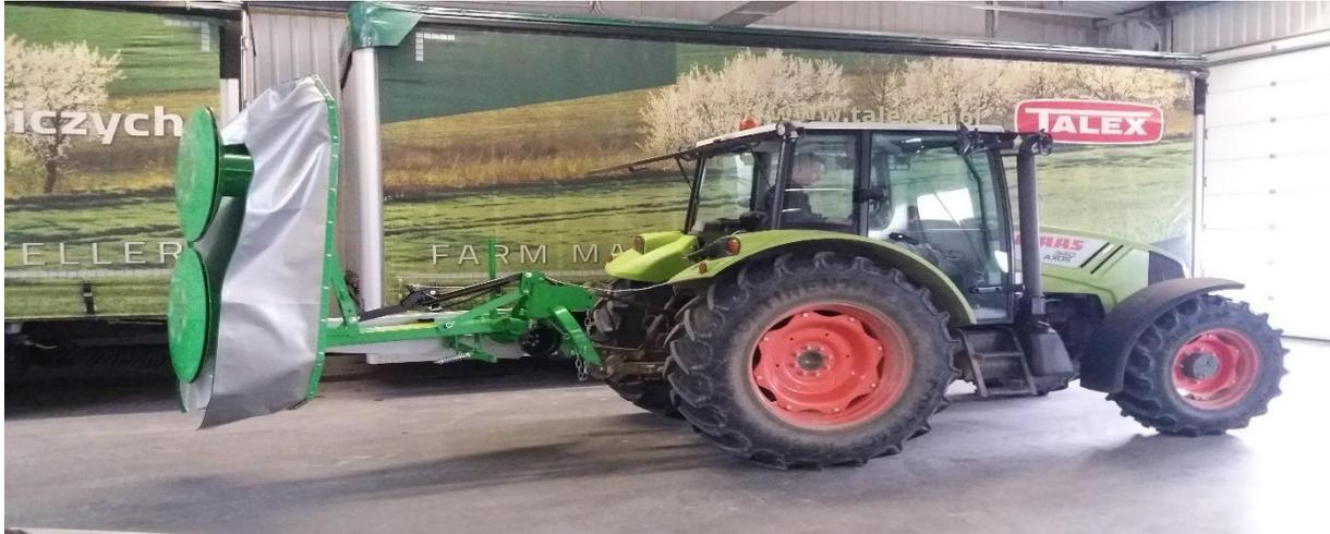
Figure 14 Proper transport position for 2.10m, 1.85m, 1.65m and 1.35m mowers with hydraulic cylinder
