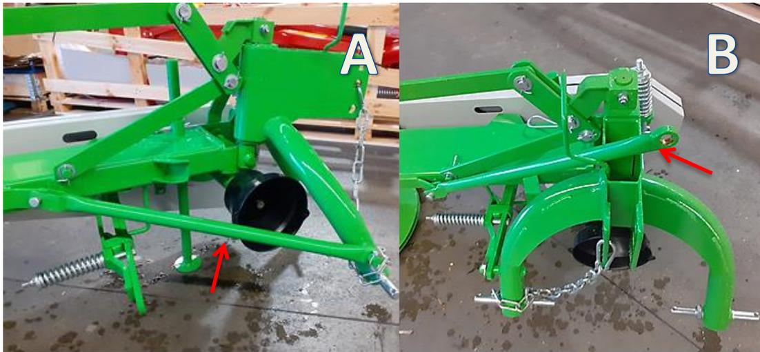
Figure 10 Transport and working position for a 1.35 m mower
