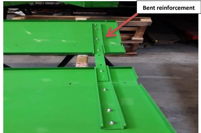
Figure 28 Step II bent reinforcement assembly
