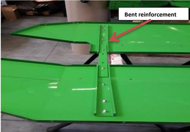
Figure 27 Step II Bent reinforcement assembly
