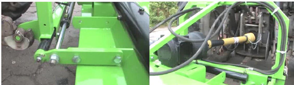
Figure 2. LEOPARD shredder – hydraulic shift of the machine
