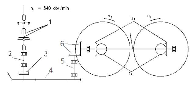
**Figure 3 Drive system diagram:** 1 – articulated telescopic shaft; 2 – drive head shaft; 3 – freewheel clutch (on large pulley); 4 – V-belt transmission; 5 – main frame shaft; 6 – bevel gear; n1 – rotational speed of tractors PTO; n2 – rotational speed of drums (values given in Table 2); z1 – large bevel gear; z2 – small bevel gear.
