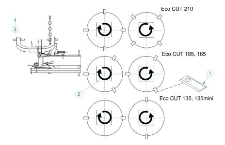
Figure 25 Diagram of the proper mounting of holders and blades on the working discs: 1) Cutting blade,
