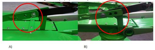
Figure 8 Proper mounting of the hydraulic cylinder in the scythe-connector: A) mower 1.85m and 1.35m with hydraulic cylinder; B) mower 1.65m with hydraulic cylinder
