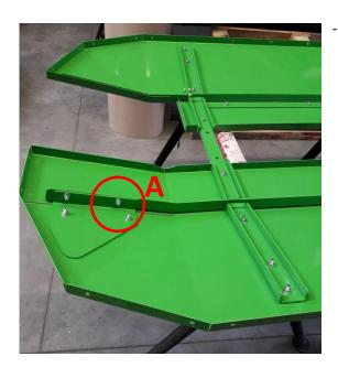
Figure 33 Step V Right cover connection
