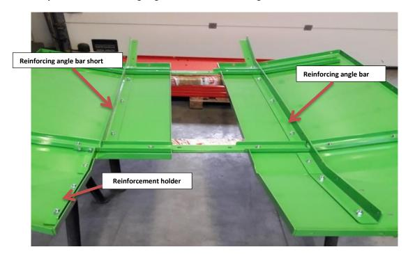
Figure 30 Step III Reinforcing angle bars assembly
