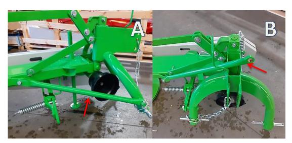
Figure 10 Transport and working position for a 1.35 m mower
