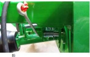
Figure 13 Suspension frame locking pin: (A) inside the clevis hole (B) removed from the clevis hole
