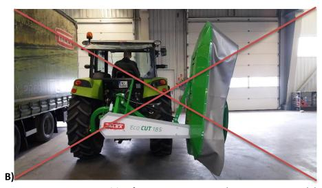
Figure 17 Incorrect transport position for 2.10, 1.85, 1.65 and 1.35 mowers, models with a hydraulic cylinder (transport position width greater than allowed by law).
