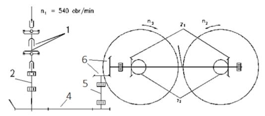
**Figure 4 Eco CUT 210 drive system diagram:** 1 – articulated telescopic shaft with one-way clutch; 2 – drive head shaft; 4 – V-belt transmission; 5 – main frame shaft; 6 – bevel gear; n1 – rotational speed of tractors PTO; n2 – rotational speed of drums (values given in Table 2); z1 – large bevel gear; z2 – small bevel gear.
