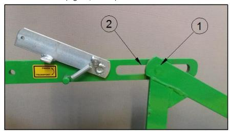
Figure 18 Proper positioning of the mower
