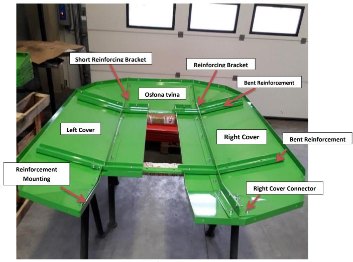
Figure 37 Step VII Checking for correct assembly
