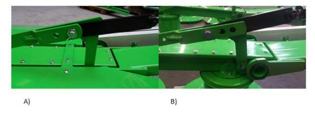
Figure 42 Proper mounting of the hydraulic cylinder in the scythe-connector: A) mower 1.85m with hydraulic cylinder; B) mower 1.65m with hydraulic cylinder
