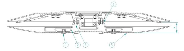
Figure 19 Cutting height adjustment: H) cutting height
