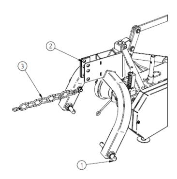
Figure 9 Aggregating – connecting the mower
