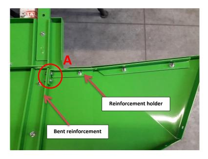
Figure 31 Step IV Reinforcement holder assembly
