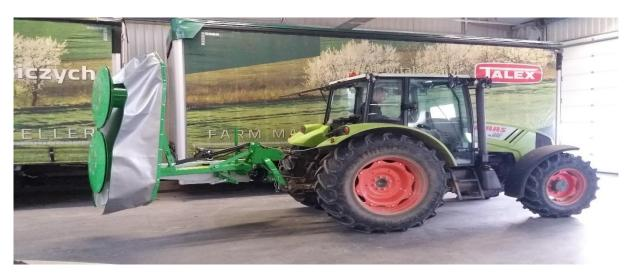
Figure 14 Proper transport position for 2.10m, 1.85m, 1.65m and 1.35m mowers with hydraulic cylinder
