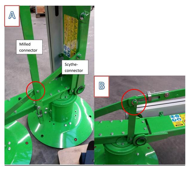
Figure 6 A) B) Assembly of the mower
