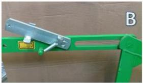
Figure 11 Interlock: transport position/working position
