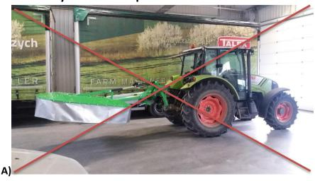
Figure 16 Incorrect transport position for 2.10, 1.85, 1.65 and 1.35 mowers with a hydraulic cylinder
