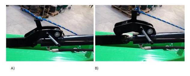
Figure 15 Locking the cylinder: A) locked, B) open
