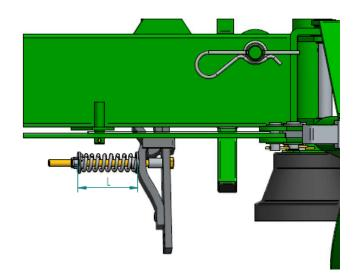
Figure 21 Break-back device - initial tension of the spring
