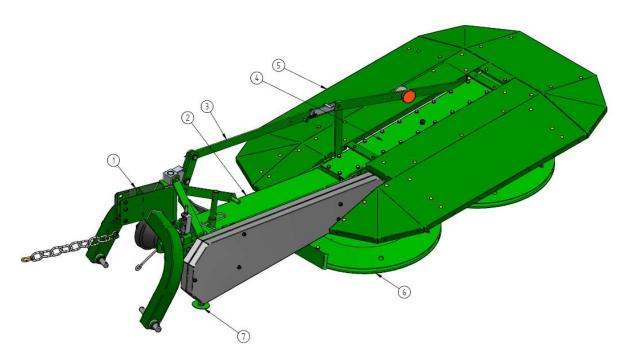
**Figure 2 Overall machine construction:** 1 - suspension frame; 2 - main chassis; 3 - connectors unit/cylinder (depending on the model); 4 - cutting unit; 5 - cover assembly covers; 6 - working section of cutting unit; 7 - support foot.
