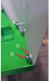
Figure 38 Step VIII Protective apron assembly
