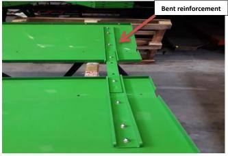
Figure 27 Step II Bent reinforcement assembly
