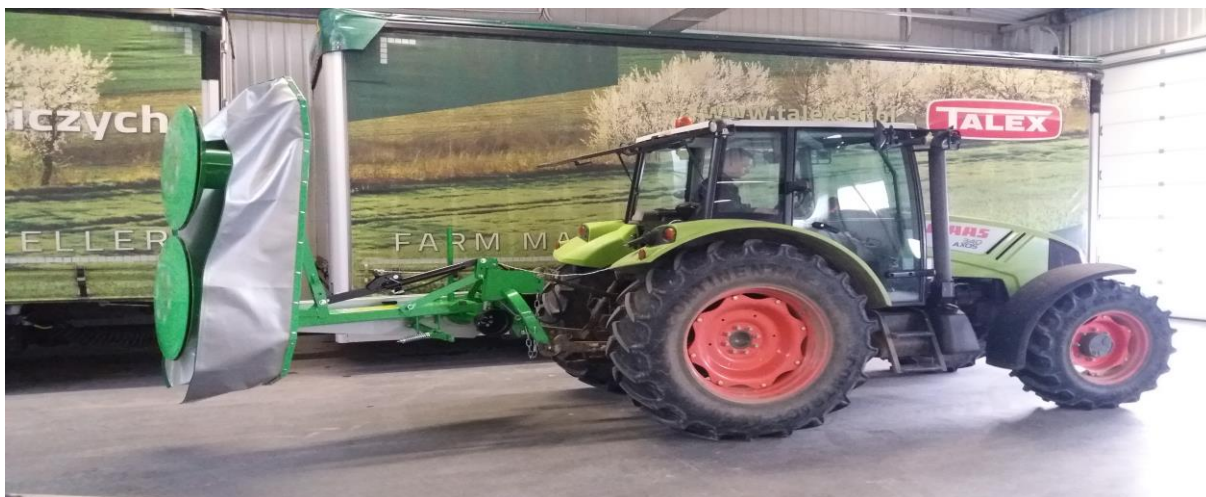
Figure 4 Proper transport position for 2.10m, 1.85m, 1.65m and 1.35m mowers with hydraulic cylinder
